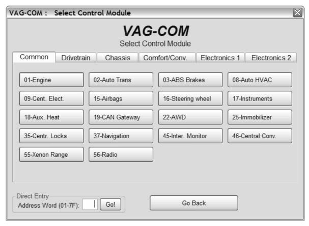
The various computers in the car are called "Control Modules" or "Controllers". On this screen, you select which Control Module you want to "talk" to. To establish communications with a particular Control Module, simply click on the appropriate button. For example, click on the button for [01 - Engine] to connect to the engine controller. VAG-COM has buttons for all control module addresses currently supported by the VAS-5051 and VAS-5052 factory diagnostic tools.
