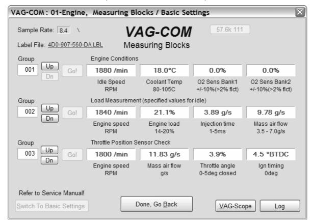
On this screen, you can read all sorts of data from the Control Module in real-time.
