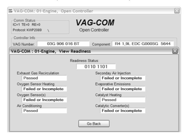
The Readiness Code is a set of 8 bits, each of which corresponds to one monitored emissions "system" in an OBD-II car. When all readiness bits show "pass", it means that all systems have been checked and that they pass the on-board tests.
