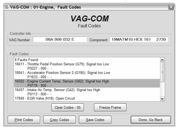
On this screen, VAG-COM shows you any DTC's ("Diagnostic Trouble Codes" or Fault Codes). VAG-COM shows the DTC numbers and also decodes each DTC into meaningful text.
