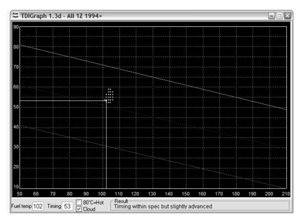
This plug-in allows you to check the injection timing setting on a TDI engine. This needs to be done after you changed the timing belt and every once in a while to keep tabs on belt stretch and pump/pulley misalignment. The standard procedure for this is to have the engine idling at operating temperature (coolant temp >85\*C), go to measuring block 000 for the engine, switch to basic settings and report fields #2 (injection timing) and #9 (fuel temperature) on a special graph.
