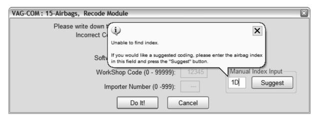
**Long Coding.** This function is needed to Recode some control modules (especially Gateways) in the newest cars that use CAN for diagnostics. Due to the complexity of Long Coding strings (up to 255 bytes of hexadecimal data) we've accommodated (and urge) the use of Copy & Paste in this function:
