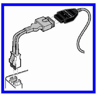
■ If your vehicle has a 2x2 port (some pre-1996 vehicles), then use the optional 2x2 Adapter between the Interface and the ports in the car.
