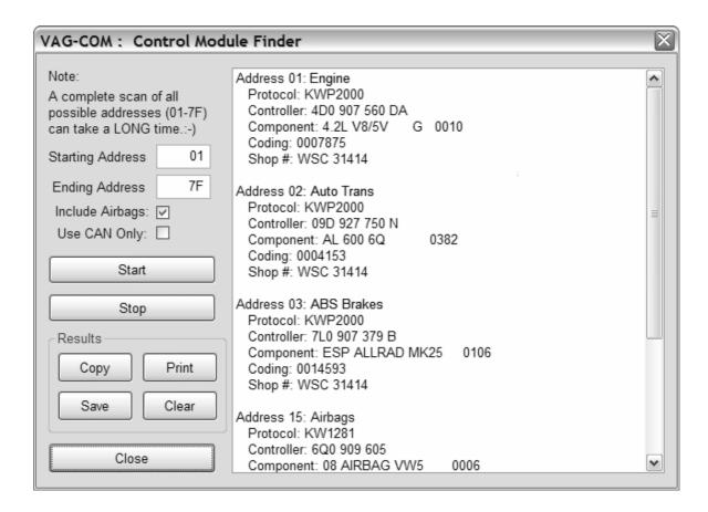
This function cycles through each possible address in the vehicle, finding each controller and reporting its Address, Protocol, Controller VAG Number, Component Number, Soft. Coding, and WorkShop Code.
