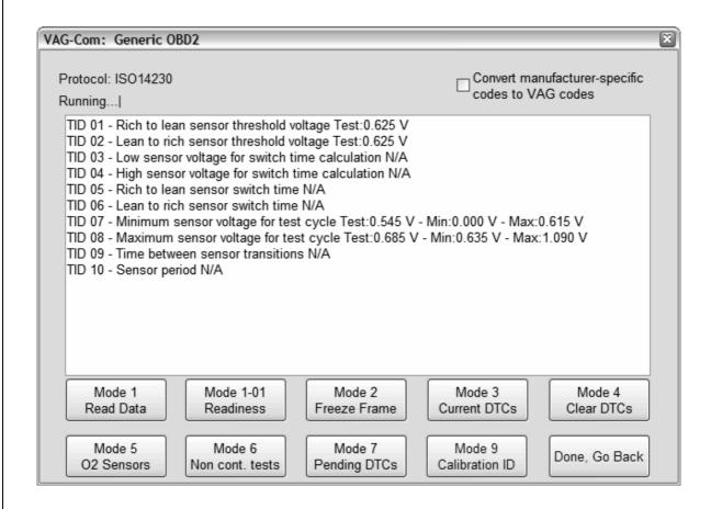
**Generic OBD-II functionality.** Because many of VW's recent factory repair manuals no longer have traditional 01-Engine "On Board Diagnostic" information and have replaced it with "Generic Scan Tool" data, this has become much more important than it was in the past. For now, we'll let the screens speak for themselves. Click each of the Mode buttons to for each OBD-II function.
