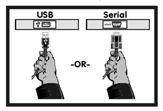
▲ Connect the Serial end of your Serial Interface or the USB end of your USB Interface to the correct port on your PC. If your PC is further from the vehicle than 6 feet, connect an approved Extension Cable between the PC and the Interface.
