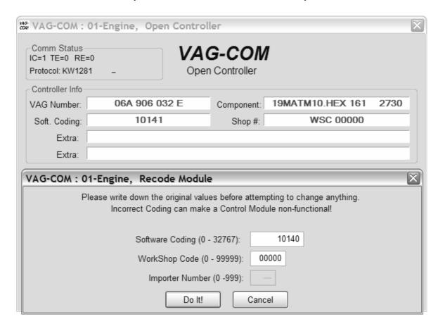
Recode is used to set various options in a Control Module.
