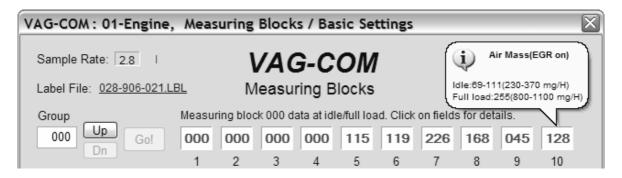
Label Files also allow a third label field to be defined for each of the normal measuring block fields. This label is displayed in a balloon when the user clicks on the field. The idea is to put "specified values" in this field:
