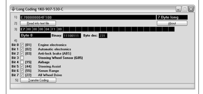
Use the **[Transfer Coding]** button to send the coding from LCode to the New coding section of the Long Coding Screen,
