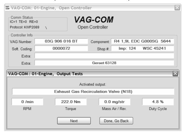
The Output Tests function is used to test a Control Module's Electrical Outputs (and the wiring that connects it to the various devices). Output Tests under KWP-2000 includes simultaneous measuring data when available from the control module in question.
