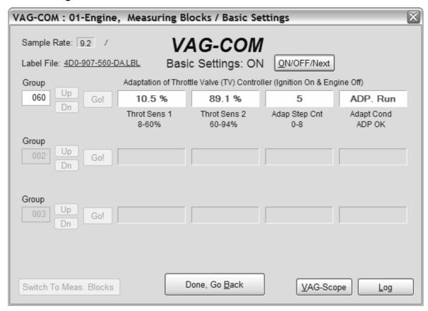
On Controllers using KWP-2000, there is an **[ON/OFF/Next]** button that allows you to initiate and exit Basic Settings while still being able to see the values in the measuring groups.
