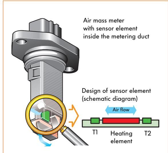
The heating element warms up the air above the glass membrane.
