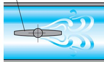
Turbulence during valve control
