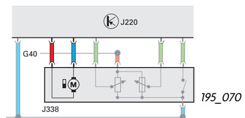
V60 is activated by the engine control unit.
