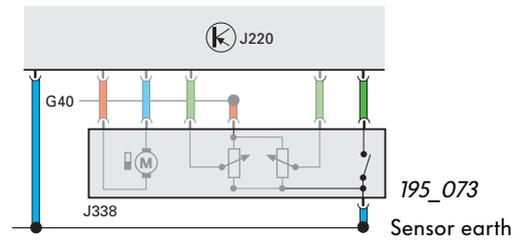
The idling switch utilises the sensor earth of the engine control unit.
