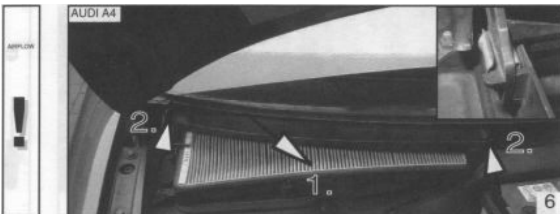
Step 6: Insert new dust/pollen filter. Reinstall water-catch trim piece by sliding it towards the windshield. Make sure it seats fully in both clips (see inset photo). Reinstall remaining trim pieces.
