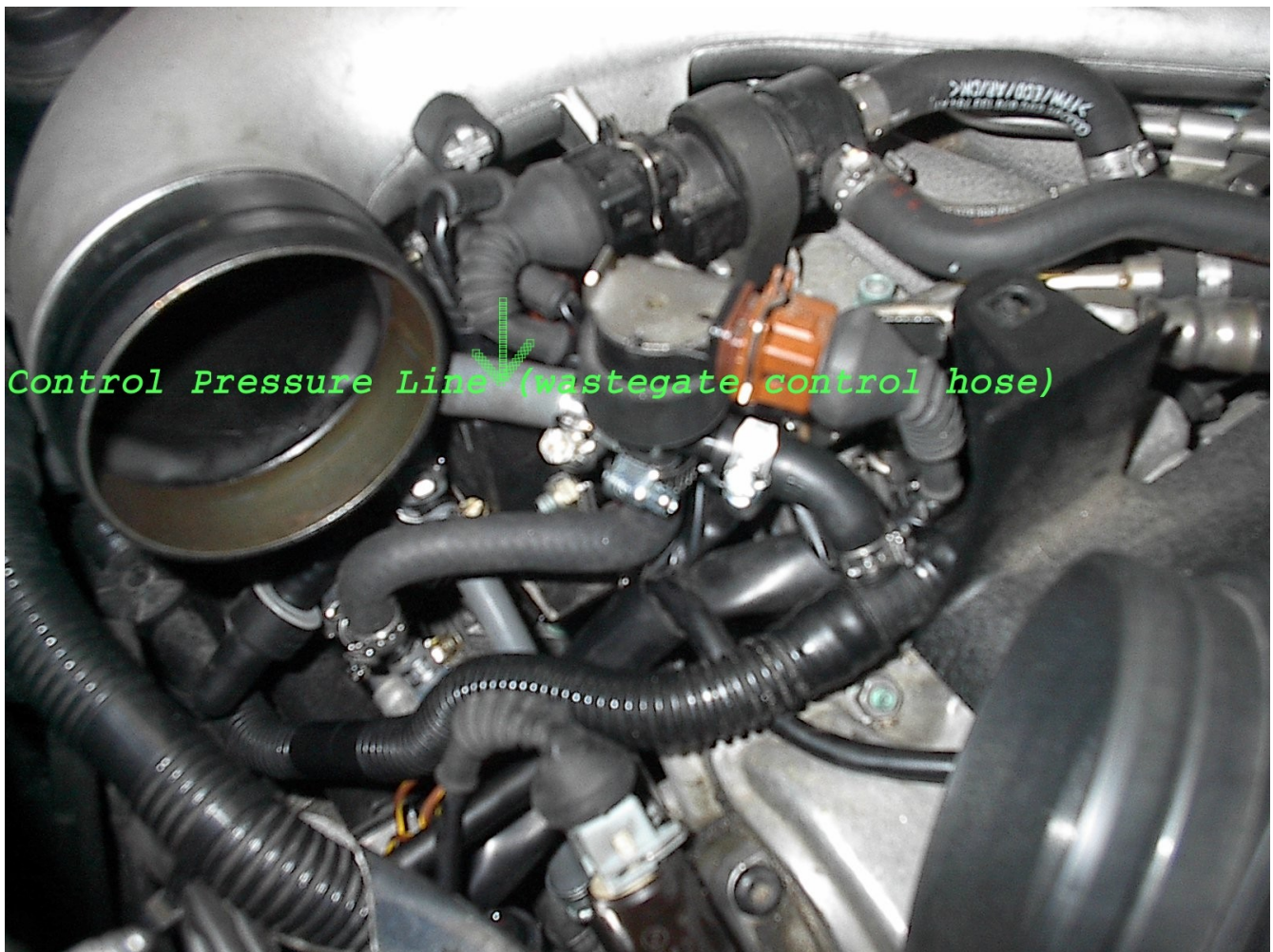
Illustration 7: Control Pressure Line (Wastegate Control)
