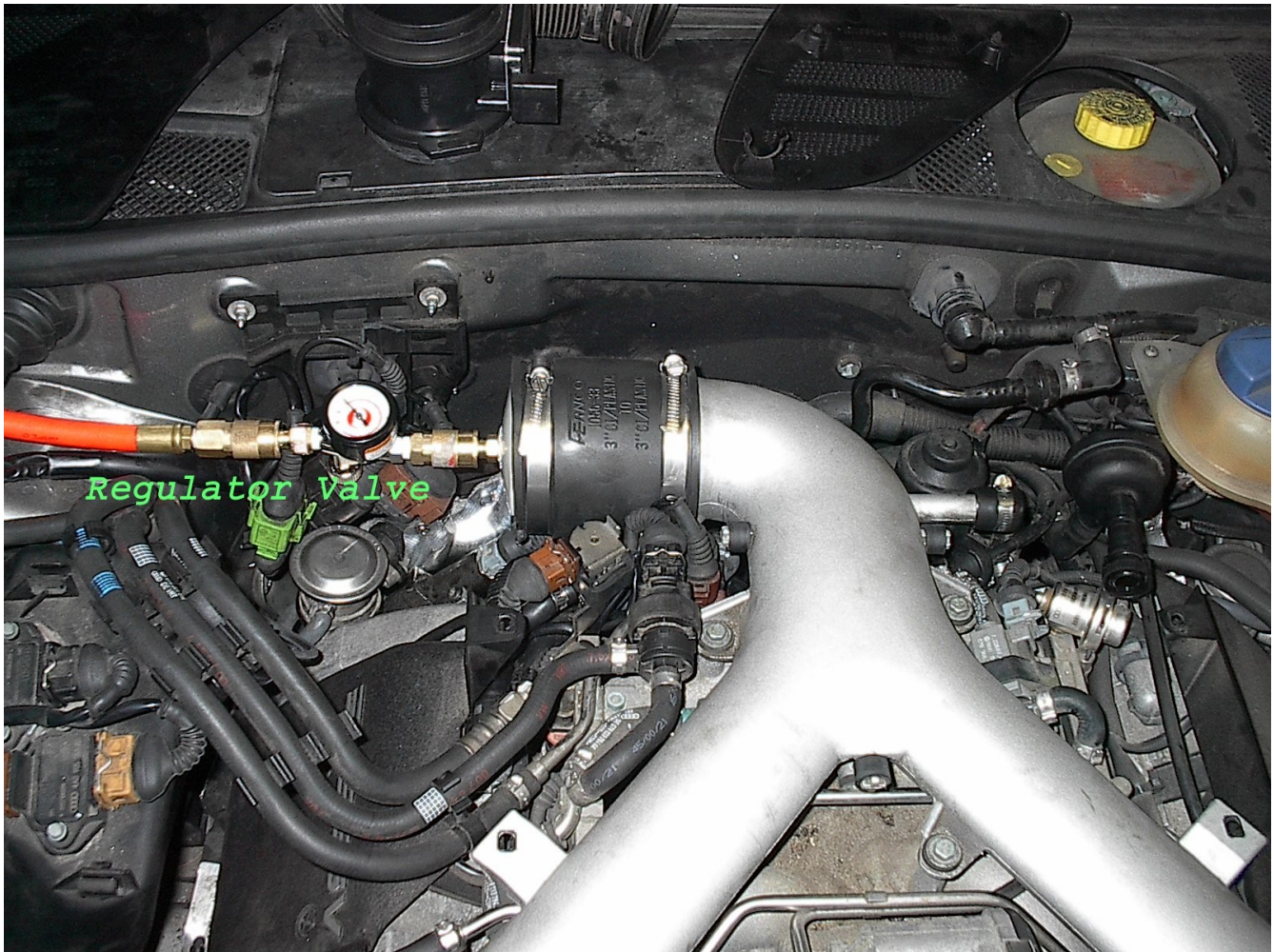
Illustration 6: Test Rig with Regulator
