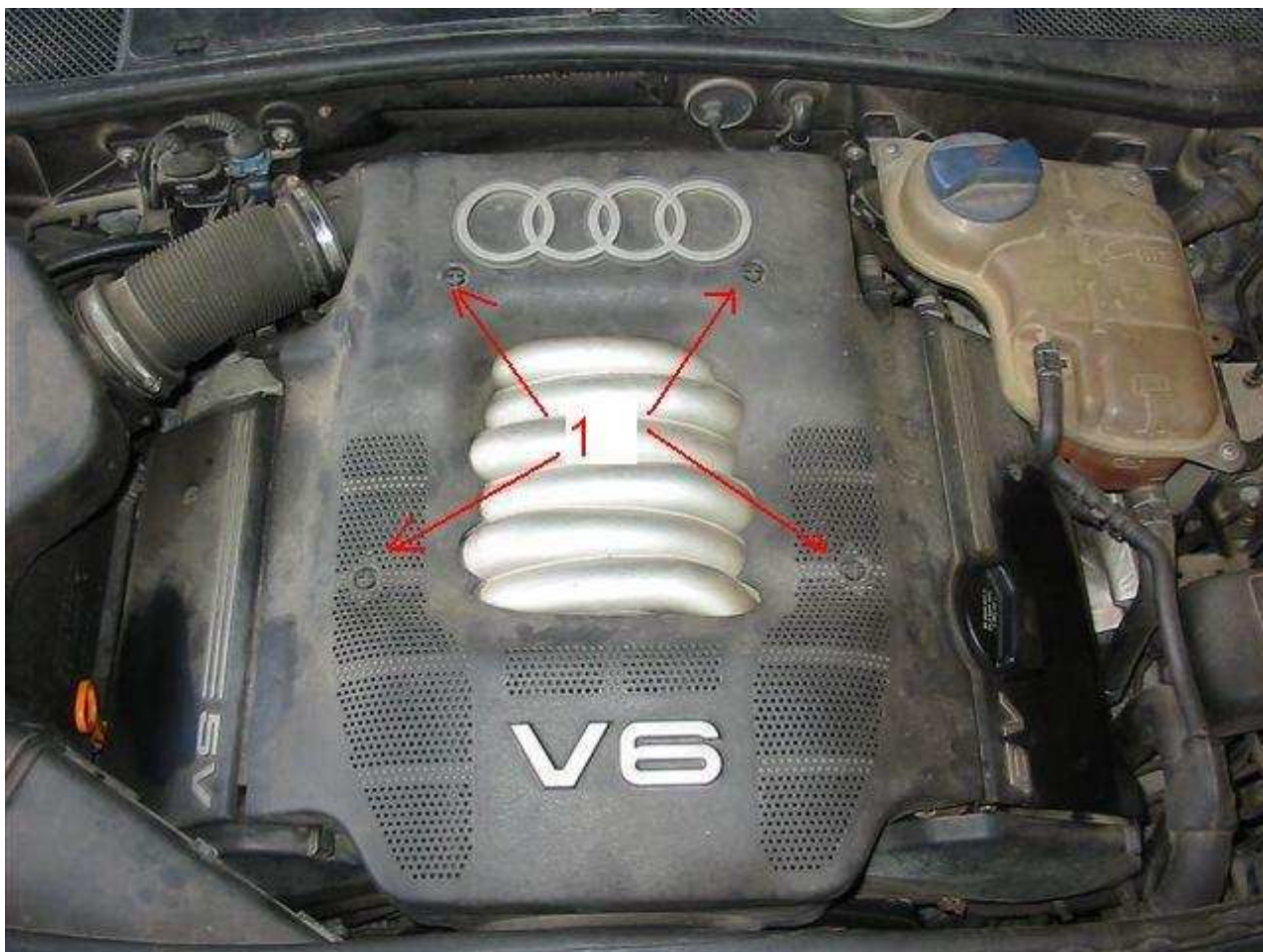
Turn 4 screws (1) 90 degrees to either side to pop up, and lift the cover
