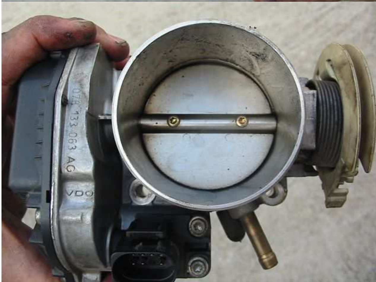
This is how it looks inside throttle body. Some oil residues and some carbon buildup was found, but in my opinion not enough to create problems
