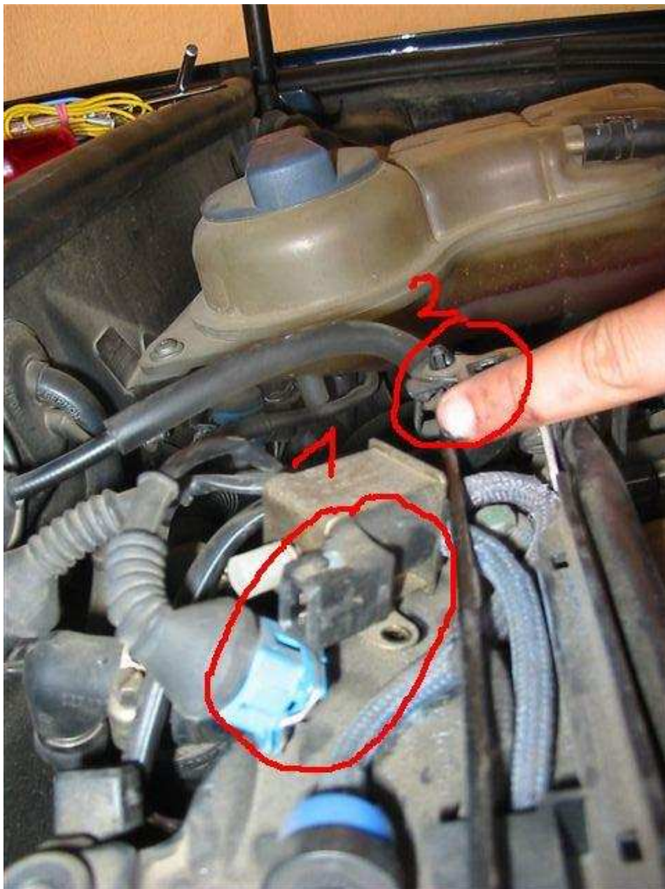
Disconnect connector (1) from vacuum valve, release the thin pipe from its holder (2) and lift mounting to the left side. Be careful as vacuum pipes are made of VERY thin rubber.
