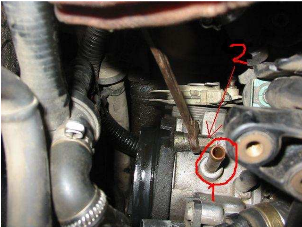
Remove tank purge pipe (1), shown already removed, and undo 10mm screw holding throttle body.
