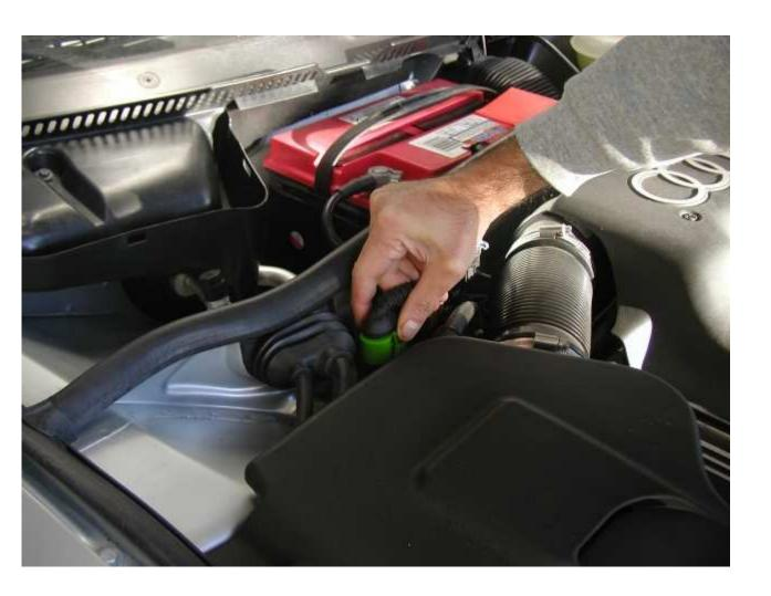
The side with the pins is connected to sensor, and the other side is wired to the ECU.
