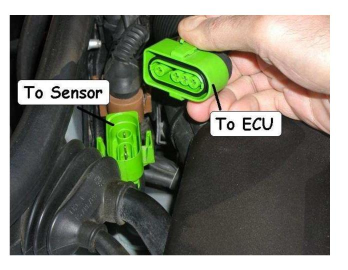
Locate pins 1 and 2 on the sensor side of the connector (these pins are wired to the sensor's heating element, pins 3 and 4 are used for the sensor's oxygen level signal).
