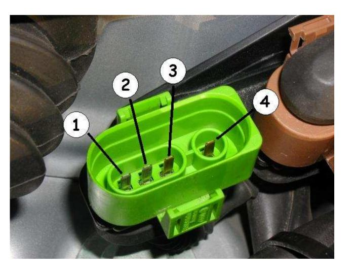
Set the multimeter to read resistance (ohms) and measure between pins 1 and 2.
