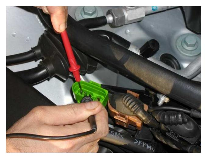
A reading below 20 ohms (as shown in the photo) indicates that the sensor heater is okay. However, a reading of 20 ohms or more (usually a lot more) indicates that the sensor is defective and needs to be replaced.
