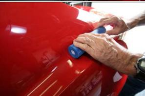
11. The concave section where the roof meets the qter panel on a lot of bodies is where this foam block shines. As seen it fits perfectly on this Big Brother Vette.
