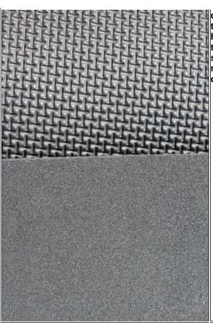
do 40 to 80 grit work, the adhesive from the paper will tend to release on to the rubber if left on too many hours. On the smooth rubber the glue residue is easier to clean off using thinner and a scuff pad or other solvent between rounds of use. It is always best to remove the sand paper on your blocks at the end of the day for less maintenance and cleanup.
