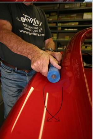
12. Another angle shows the rotation needed to achieve the results "black arrows". Twist your fingers in this direction while moving your arms back and forth on the panels, 18-24 inch long strokes. Everything is done in criss cross patterns. The difference is how long the stroke is and how tight the criss cross is done.
