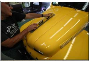
screw the lexan to and then apply the rubatex rubber. You have a dead on straight surface with this fabricated block.
