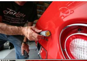
13. These duro blocks are a tiny open cell rubber material. It "gives" a little bit meaning it tends to move with the panel. As seen Bill is using it against the taillight panel on this Vette as it fits nicely. It works well in all grits from 40 to 2500 color sand work. We cut them to different lengths in order to fit them to our panels. We also round the edges a bit to keep them from digging in.
