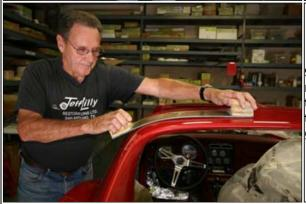
9. This flex block can be used in a myriad of places but roofs or sloping areas where you want as much contact to the surface as you can get is most important. With the thin 1/8th lexan it is best suited when doing 180-400 grit work like primer blocking.
