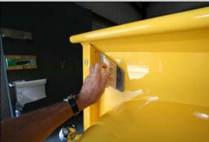
23. Up inside the bed we used an angled block we fabbed to fit in the corners. This enables you to block with out digging a rut or valley when trying to match the inside edges.
