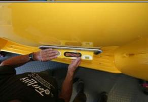
24. Large panels like this convex door require a simple flat block 18 inches long. We have 11 inches of contact in the middle. This type of shape is gravy or easy to perfect. Notice the hand and fingers. Just enough pressure that you do not push against the panel and your hands will not become fatigued easily. The vehicle should not rock and or move at all or you are being to aggressive and pushing which will tend to dip the surface.
