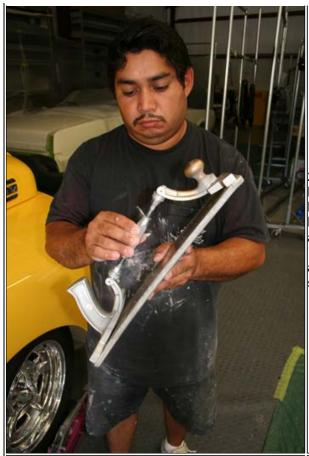
20. Nat Ramirez shows us a double wide adjustable block we fabricated. Using an adjustable lead file we built this block to use on panels requiring heavy duty blocking. Just twist your fingers till your desired fit against the panel you are working and your ready to "block and roll". Nat is the best blocker I have ever seen and can remove any ripple or imperfection on any body style thrown his way.
