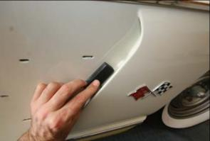
18. Many square shapes can be cut from the open cell Durablock rubber to fit a section. As with this inside panel we needed to finish it off for no flaws. We chose a piece thick enough for our fingers to hold it steady yet thin enough to fit inside and clear the overhang.
