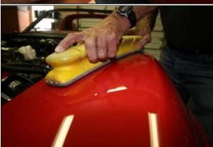
15. This foam block works good when going from a high to a low section. We removed the rods which stiffened it too much in our opinion " black arrow" These ran through the length of it. We then sliced the foam top, half way down to make it flex side ways and front to back like a "centipede" if you will. Eastwood sells a model like this one but they need to be modified for optimum results much like what we did to this one.
