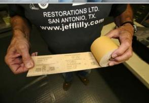
6. The 3M gold stikit paper is the choice to use when sanding primers and fillers. 80 to 500 grit while refining and sculpting. When doing body filler work 3M 40 Board Files # 2231 only come in 17 inch strips. Here are the following part numbers for the continuous rolls.
