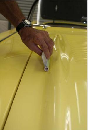
19. 1/2 inch pvc makes a great block with a glued on handle to grab while blocking. This works great for tight areas like where the spear drops off in to the flat area of this hood..
