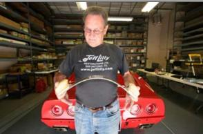
8. With 51 years of blocking experience Bill Lilly qualifies as an authority on the subject. Here he demonstrates one of the flex blocks, notice how easy this block flexes. Two fingers on each end allows ample pressure to get it moving. This block was made from two 3M yellow hand blocks on each end and an 18 inch long piece of 1/8th thick lexan double wide for two sheets of stick it paper. Rubatex rubber was applied with contact cement.
