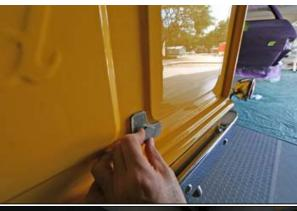
22. The rounded corners of this tail gate show a lexan mini block made specifically for this panel to get the results needed. As seen the tail gate shows its reflection stuff revealing the proper tool was used. You can purchase lexan at a plastic supply house in any desired thickness. Simply cut it with a jig or band saw and then file the edges burr free. Drill, taper, screw to a hard level or straight block then add rubber and you are ready.
