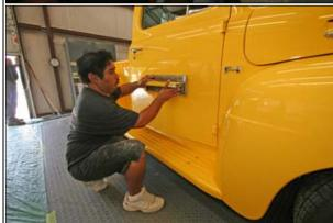
25. The holding of a block is equally important for the criss cross pattern needed to achieve the best results " see arrows " Nat is in position with the "Body mans crouch" balanced and ready. We also use rolling office chairs while working some panels if access is available to the panel. In this case the running board would not allow him to sit in a chair while blocking.
