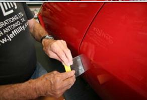
14. When perfecting gaps we use small metal spreaders 1 to 2 inches wide as seen. Too wide and it tends to dig on the ends as you are working a gap. Too narrow and it does not keep a straight line. These two sizes work best. Simply wrap the stick-it sand paper around it as needed. Always work panel to panel never work a body panel off a car separate from each other or your quality will suffer.
