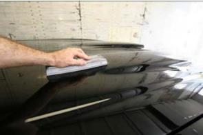
27. This Super Rod Firebird received the "Durablock" treatment with the 9 inch block to sculpt the hood scoops to the flat section for a no ripple transition. A very strange and unusual shape to deal with. "Red Line Shows It"
