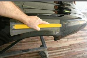
29. A different fender lip or gradual flare style used on a lot of GM cars like Camaros require a C- Block. This was cut specifically for this type of shape. It removes dips and allows you to get in to the contours as close as possible.
