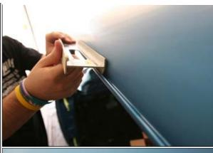
30. This skinny open level does a great job with 1/8 thick rubber, on drip rail inside edges. This is an area that needs a special block like this in order to get close inside the drip edge for a ripple free surface.
