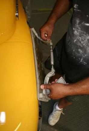
21. As seen Nat adjusted the block to fit this rounded contour on a 50 Ford Custom truck. As much surface contact as you can get is best with the ends just off the panel.
