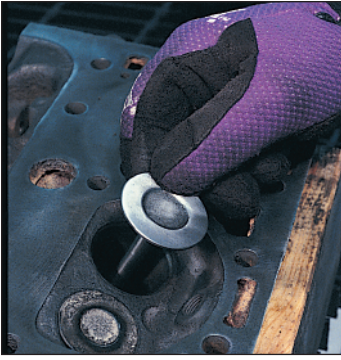
Before doing the chambers, install a set of valves to protect the valve seats.
