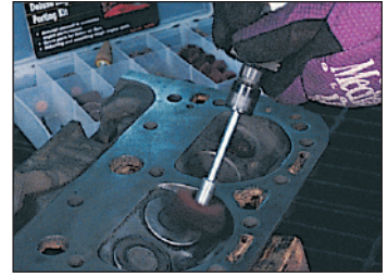
Cross Buffs are used to finish the combustion chamber.
