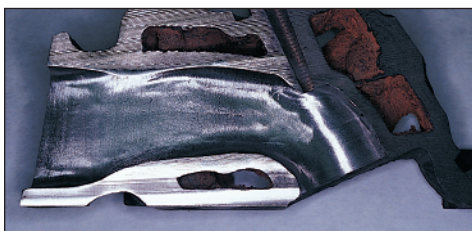
With this cutaway, we polished the whole port to better illustrate the rough-to-touch finish. Note the smoothed valve guides and short side radius.
