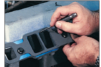
The Fel-Pro intake gasket is used again to mark the manifold. You want the top of the gasket to face the manifold whereas you had the bottom of the gasket facing the head.
