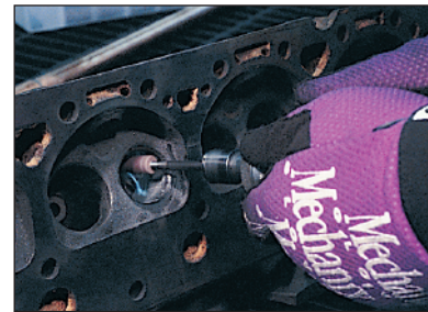
Bowl work is the second part of the basic porting. Here a half-tapered cartridge roll is used to smooth the valve guide. While this picture shows work on an exhaust port, the valve guide work is the same be it in an intake or an exhaust.
