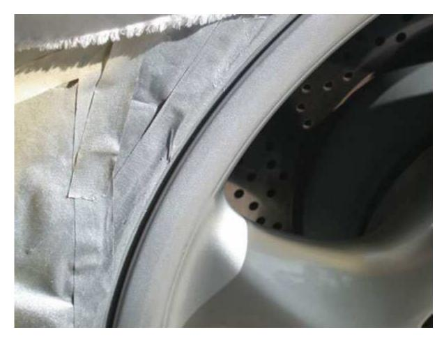
Okay, fast forward a few minutes...I had to roll the car forward a bit to keep it in the sun and I had cleaned (and let fully dry) the wheel and RE-sprayed the silver. Now I'm using the NASA technique on the silver paint and CAREFULLY removing the overspray:
