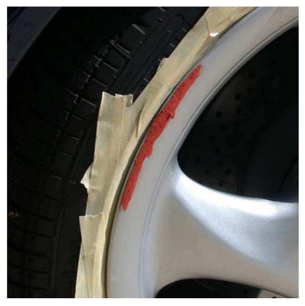
I like to START by masking the tire from the wheel...get the masking tape WELL behind the rim. Next, sand the area to a nice "feather" with 240 grit sandpaper and wipe some spot putty on. IMPORTANT...this ENTIRE project will work best if the wheel is in the sun and its a nice warm day...the drying time of spot putty is minutes but if it's cold or damp, this project is likely to not work out too well. Remember...keep your sanding to the IMMEDIATE area around the damage. Trust me on this.
