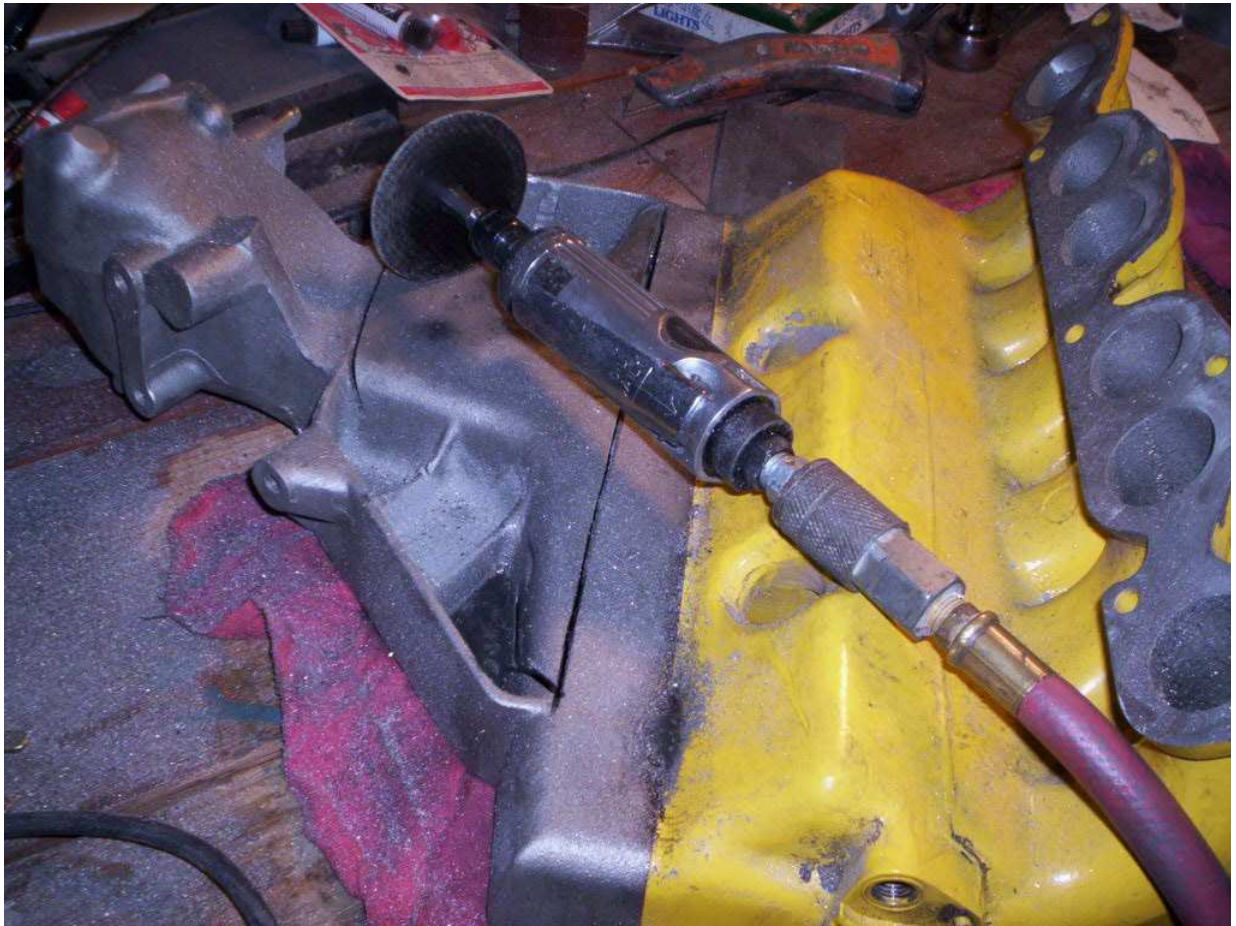
you want to cut along the top of the bottle neck to meet the 2 lines you allready cut. so you can remove the peice like so..
