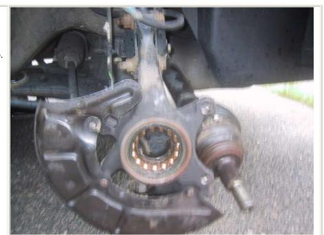
12. Use a washer that seats comfortably on the inner race, but is slightly smaller than the outer race. Place this washer on the inside of the wheel knuckle. As you tighten, you want this washer to pull the wheel bearing out of the wheel knuckle. In addition to the washer, I used several smaller washers on the inside end, threaded the nut on and pulled the bearing into the cup. The bearing will fight to stay in - apply steady pressure.
