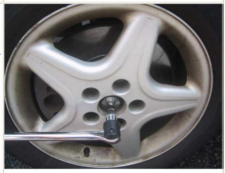
4. Jack both sides of the car up. Use jack stands in addition to your jack to ensure safety. Remove the five lug bolts. Remove the wheel from the car. The rotor and brakes will be exposed.
