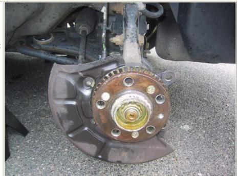
7. Remove the 30mm 12-point nut from the outer CV joint axle.
