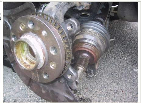
10. You'll now use the wheel bearing puller in different configurations to first remove the old bearing and then install the new one. Place the bolt through the ABS adaptor, through the wheel hub. Thread the nut onto the other size. Use an adjustable wrench on the inside nut and a 36mm socket to tighten the bolt. Place the ABS adaptor against the wheel knuckle so it is secure.
