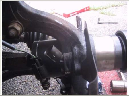
15. Picture of the new bearing installed. Now, install the new circlip (that came with the wheel bearing kit - don't use the old circlip). Again, using the needle nose pliers, squeeze the circlip and it will snap into place (in the groove of the wheel knuckle) to secure the bearing. You may need an extra pair of hands to push while squeezing the circlip in.
