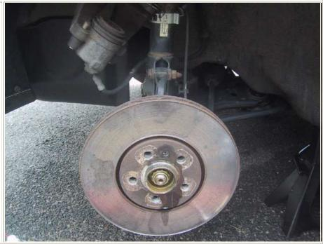
6. Notice the single Phillips screw on the rotor. Unscrew this screw and remove the rotor. The screw may be rusted and seized and will need to be drilled out. The rotor may be rusted and sized to the wheel hub. You may need to hit it (very hard) with a hammer (and WD-40) to get it off the wheel hub. This picture shows the wheel hub after the rotor is removed.
