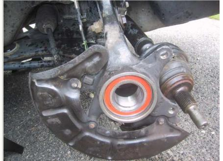
16. Push the new wheel hub into the inner race. Use an washer on the side that fits into the inner race, but is slightly smaller than the outer race. Thread the bolt through the wheel hub, through the bearing and attach the nut. As you tighten, it will press the hub into the bearing.
