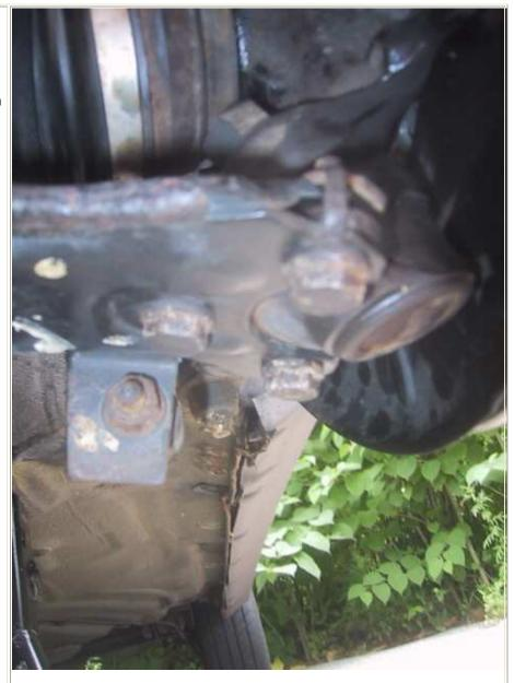
9. Remove the wheel hub and wheel knuckle from the outer CV axle. Push the axle into the hub. You may need to hit it with a hammer if it is rusted. If it is badly seized, barely thread the nut back on and use the hammer to hit the nut - in this way you won't damage the axle threads. The picture shows the axle free of the wheel hub once the knuckle has been swung out.
