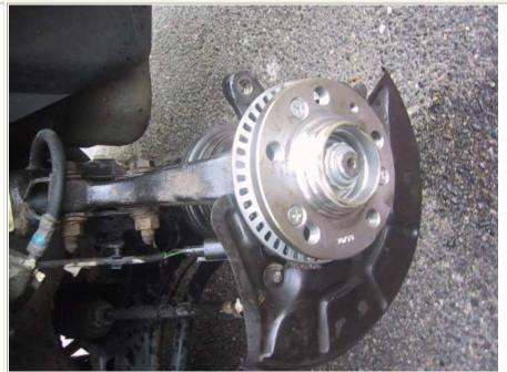
18. Place the rotor onto the new wheel hub. Insert the philips screw to hold the rotor onto the hub.
