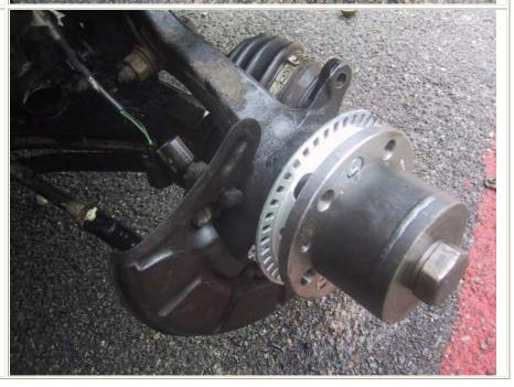
17. Insert the CV axle into the new hub.
