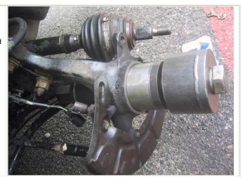
14. Second picture of pushing the new bearing in. On the inside, we're using the cup with a washer and the nut. Note that I've removed the ABS sensor wire so it isn't damaged.
