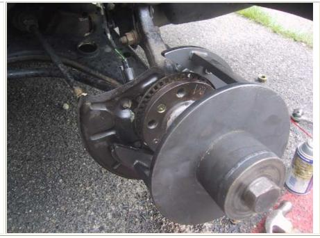
11. As you tighten, the wheel hub and inner race of the wheel bearing will come off. Notice that this wheel bearing has failed (see rust colored bearings). Before you can remove the rest of the bearing, you must remove the circlip. The circlip keeps the bearing in place; it is a metal ring that fits inside the wheel knuckle against the bearing. It has two holes. Use the needle nose pliers to squeeze the circlip and remove it.
