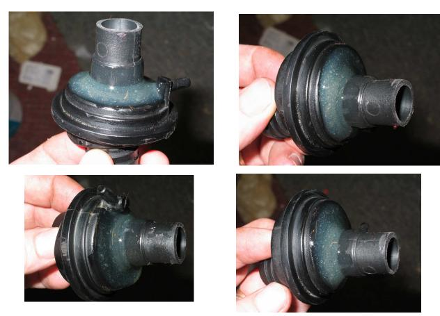
Eventually I put it back in the vice, but upside down to set (below). You can see the epoxy is nice and thick around the base of the connection, where most of the strain would be.
