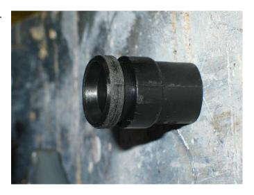
Test fit cut connector to valve body. I scuffed the edges of the new connector a little to help the bond. Also scuff the top of the valve to help the epoxy get a good grip (did this on my on second attempt not in the picture
