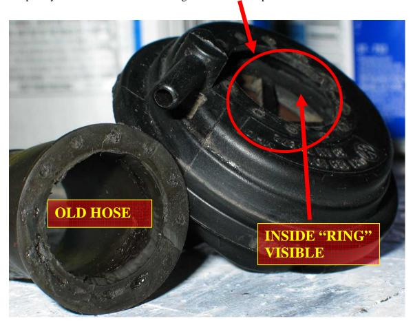
Then remove the inside ring of the old hose. The picture (above) "barely" shows it. Below it was removed. (sorry no pics of the removal). I used a pair of thin long nose pliers to break the plastic "ring" it into smaller pieces to pulled them out. MAKE SURE YOU GET ALL THE PIECES!!! YOU DO NOT WANT THESE TO GET INTO THE INTAKE MANIFOLD. WILL NOT BE GOOD IF THEY GO THROUGH THE MOTOR!!!
