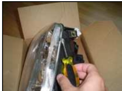
Remove top clips gently with screwdriver.
