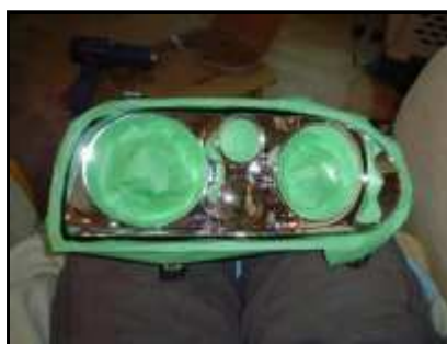
Final masked product, I also taped off the seal so I could reuse the existing silicone.
