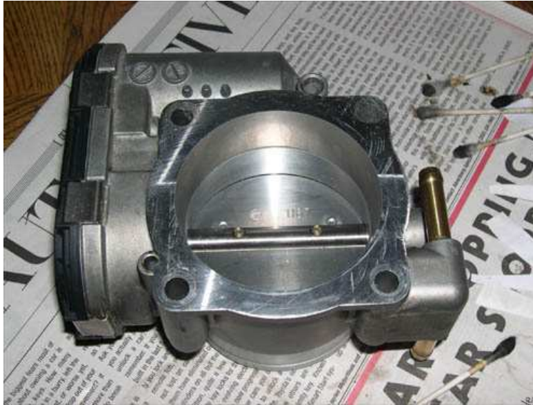
9. The pictures below of paper towels and Q-tips used during the cleaning procedure illustrate that while the TB did not look that dirty, quite a bit of deposits were removed during the cleaning process.
