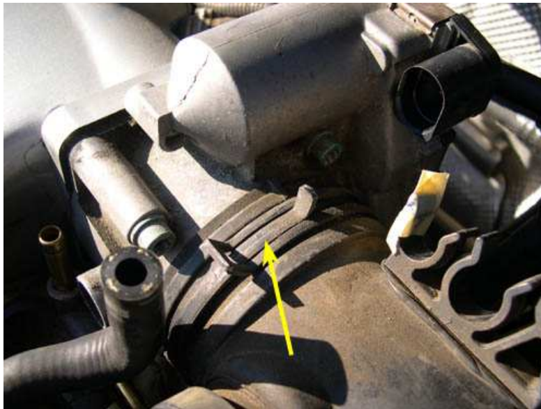
27. The picture below shows the large amount of condensed oil vapor in the main intake tube due to the PCV circuit. I wiped this oil off the inside of the tube with a paper towel. (I can only imagine how much oil is in the intake manifold and elsewhere in the engine. Someday I'll clean it all out.)
