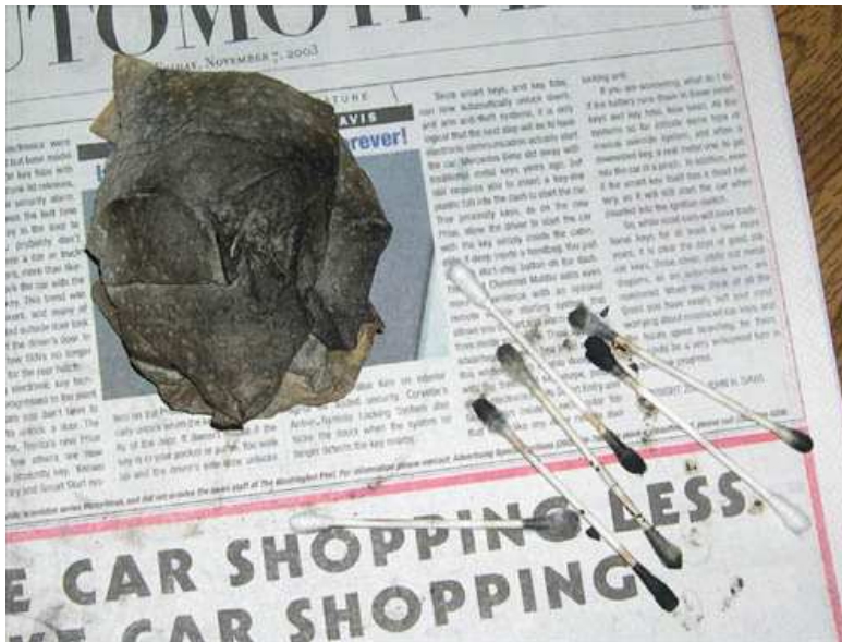
9. The pictures below of paper towels and Q-tips used during the cleaning procedure illustrate that while the TB did not look that dirty, quite a bit of deposits were removed during the cleaning process.
