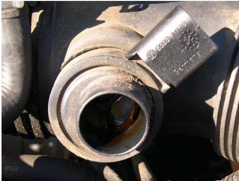
23. Disconnect the upper coolant hose (yellow arrow in picture below) from the TB. The nipple on the TB is approximately 1" long, so the clamp has to be moved up the hose at least that much in order to remove the hose from the nipple.
