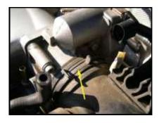
Release the tension from the clamp securing the main intake tube to the TB (indicated by yellow arrow in picture above) and then slide the intake tube off of the TB.
