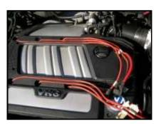
Unclip the spark plug wires from the channels in the engine cover, as shown above.
