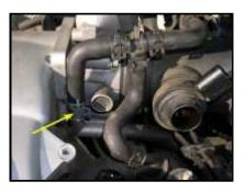
Disconnect the upper coolant hose (yellow arrow in picture above) from the TB. The nipple on the TB is approximately 1" long, so the clamp has to be moved up the hose at least that much in order to remove the hose from the nipple.
