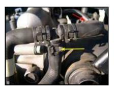
Disconnect the vertical coolant hose (yellow arrow in picture above) from the T-junction in front of the TB/main air intake tube. Next, unclip the horizontal portion of the coolant hose T-junction from the top of the main intake tube (red arrow in picture above) and then move the hose out of the way. At this point, there should be no coolant hoses attached to the TB, nor should there be any coolant hoses or electrical leads passing over the top of the main intake tube.
