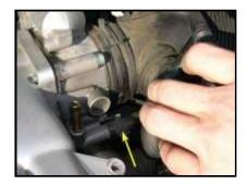
Disconnect the lower coolant hose (yellow arrow in picture above) from the TB. Again the nipple on the TB is approximately 1" long, so the clamp has to be moved down the hose at least that much in order to remove the hose from the nipple.
