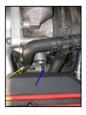
Disconnect the upper coolant hose (yellow arrow in picture above) and lower coolant hose (blue arrow in picture above) from the TB. To do this, use the appropriate tool (pliers or screwdriver) to release the tension from the hose clamp, slide the clamp down the hose and out of the way (for spring clamps, make sure the clamp is moved past the end of the nipple inside the hose or the clamp will reapply pressure to the nipple when released), and then pull the hose off of it's nipple.
