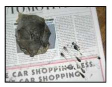
The pictures above of paper towels and Q-tips used during the cleaning procedure illustrate that while the TB did not look that dirty, quite a bit of deposits were removed during the cleaning process.
