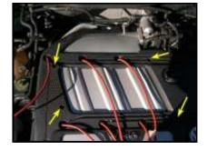
Remove the main engine cover piece by removing the four (4) T30 Torx screws indicated by the yellow arrows in the picture above. As you lift up on the cover piece, you will need to thread the spark plug wires through their respective holes in the cover in order to fully remove it.
