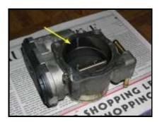
The four pictures above show different views of the inside of the throttle body. The yellow arrows in these pictures point to the oil, gum, varnish and other crap that deposits itself inside the TB over time. In my case, most of the deposits were located between the edge of the throttle valve and the TB wall (valve at idle position or fully closed) and on the roof of the TB wall behind the throttle valve.
