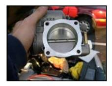
The picture above shows the cleaned TB ready to be reinstalled.
