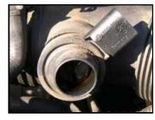
The picture above shows the inside of the PCV valve/heater on the main intake tube. If you look closely, you can see the abundance of condensed oil vapors.
