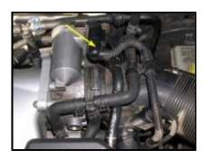
Disconnect the harness connector from the TB. The connector is indicated by the yellow arrow in the picture above.
