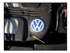
Remove the small engine cover piece with the VW logo on it by removing the single T30 Torx screw, indicated by the yellow arrow in the picture above.
