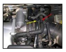
Unclip the coolant hose (red arrow in picture above) and the PCV vacuum-assist hose (yellow arrow in picture above) from the top of the air intake tube.
