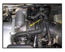
Release the tension from the clamp securing the main air intake tube to the TB (indicated by yellow arrow in picture above) and then slide the intake tube off of the TB.
