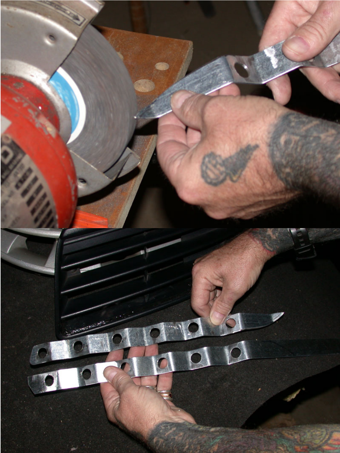
Here I am shaping the metal straps for the light bar.
