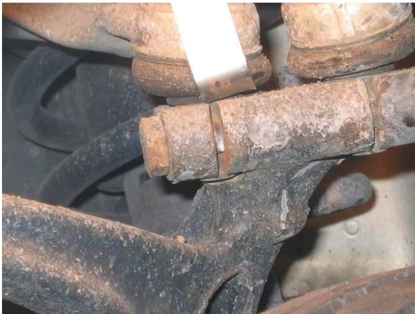
I don't know if you can see it, but look for the half cut through bolt.
