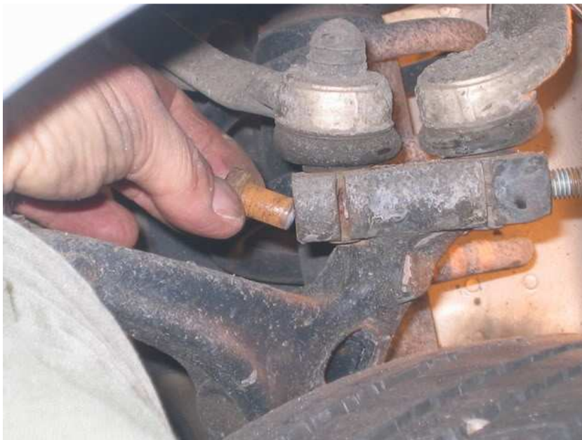
Break off half cut through bolt head with wrench, and remove.
