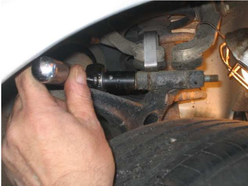
Break off half cut through bolt head with wrench, and remove.
