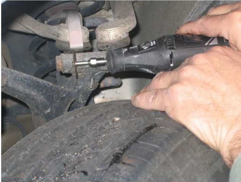
Cutting through with Dremel tool. Only cut 1/2 way through. You don't want to cut into the ball joint pin that is held in by the pinch bolt. Notice shield to protect boot.
