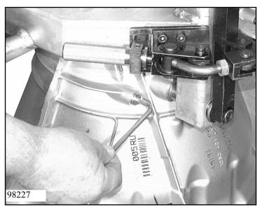
Remove all (screw) plugs from the transmission housing. Remove breather cover.
