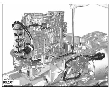
Unscrew the screw of the Hall-effect sensor and pull the wiring harness leading to the sensor out of the retaining groove.
