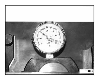
Then put measuring bar 5p01 060 330 on the measuring plate, insert the measuring base of the dial gauge into the groove of the measuring plate on the top disc of the pack and set the dial gauge to zero.
