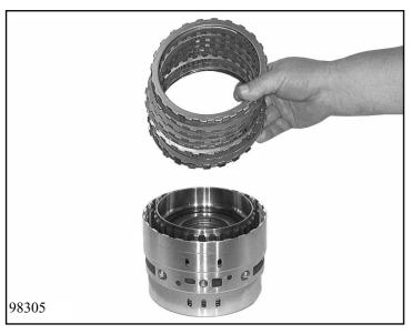
Turn the complete unit and remove the counter support.
