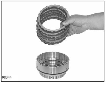
Insert complete disc pack of clutch A. Start with spring disc 70.010/190, followed alternately by outer discs 70.010/200 and lined discs 70.010/210. Add final disc 70.010/220 and secure with snap ring 70.010/230.
