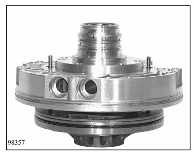
Twist 2 centering pins (M6) into the pump, place the intermediate plate over them and push in.
