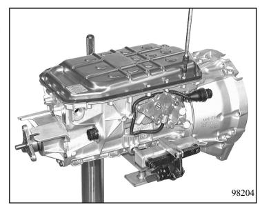
Unscrew the 2 screws used to fasten the oil filter and remove it.
