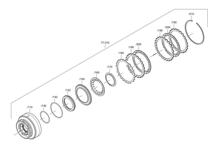
Press 2 new O-rings 77.010/130 and 77.010/140 onto piston 77.010/120 and press this into cylinder F 77.010/110. Place pressure plate 77.010/150 on piston.
