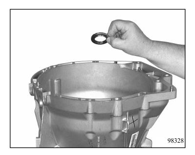
Insert sun wheel shaft 32.140 and check operation.
