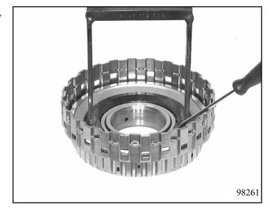
Cover one oil feed hole and force the piston out with compressed air through the other.
