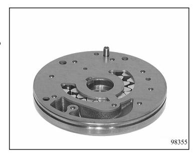
Screw 2 centering pins 5x46 001 007 into intermediate plate 10.060/110.
