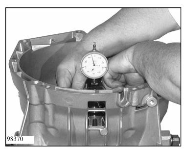
Determine axial play by pressing and pulling on the handle (repeat measurement).
