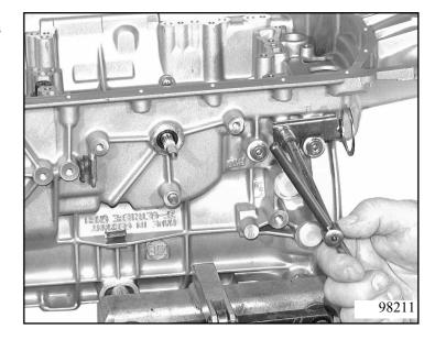
Drive the clamping sleeve out of the selector shaft and remove the selector shaft. Remove the detent disc and connector rod and release the rod from the disc. Remove the shaft seal with a suitable tool.
