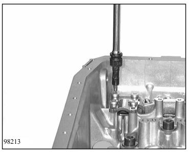
Unscrew the 4 screws of the guide plate and remove the guide plate.
