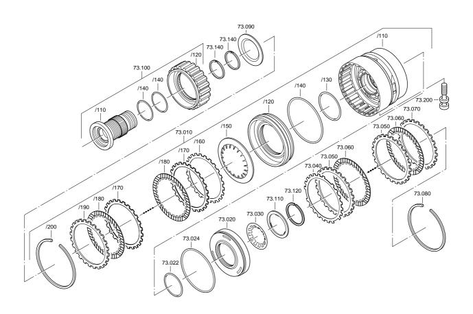
First determine the release clearance of the brakes DG.
