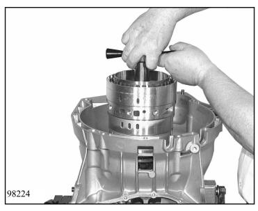
Lift out the tower and insert into holding device 5x46 002 006. Remove the shim.
