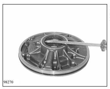
Lever out the shaft seal with a suitable screwdriver and take off the disc.
