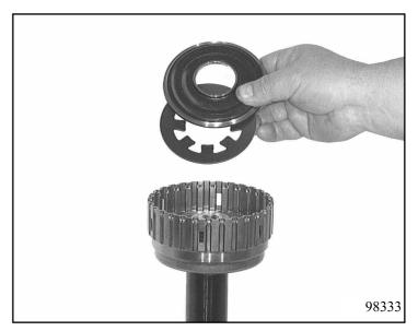
Push the oil dam down with assembly bracket 5x46 030 167 on a mandrel press and fit retaining ring 71.090 with suitable pliers.
