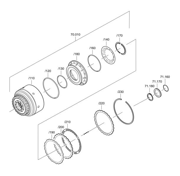
Pull new O-rings 70.010/120, 70.010/130, 70.010/160 onto piston A 70.010/180.
