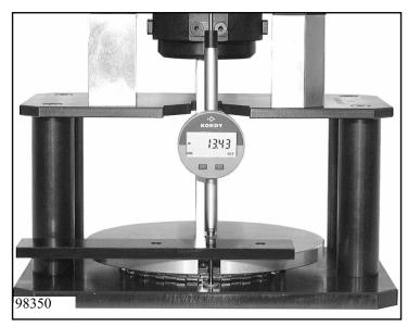
Determine thickness  $\mathbf{M}_{\mathbf{B}}$  of the clutch B disc pack according to
