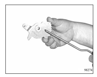
Insert the detent disc and connector rod into the transmission housing and push in the selector shaft 01.010/160.
