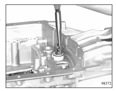
Place the complete control unit on at an angle.
