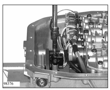
Insert inductive transmitter 27.040 in the hole provided and fasten it with 2 screws 27.060.
