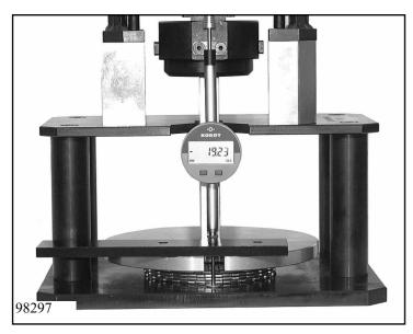
Determine thickness  $\mathbf{M}_{\mathbf{E}}$  of the brake E disc pack according to
