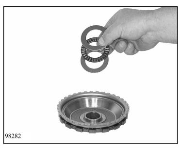
Insert thrust washer 42.070/110, axial needle roller bearing 42.070/120 and angle washer 42.070/130 into parking lock wheel 42.090.
