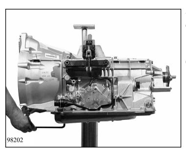
Unscrew the oil inlet/drain plug and drain off the oil.
