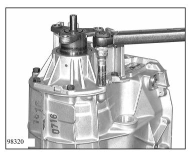
Place output assembly on and fasten with 7 hexagon screws 14.110.
