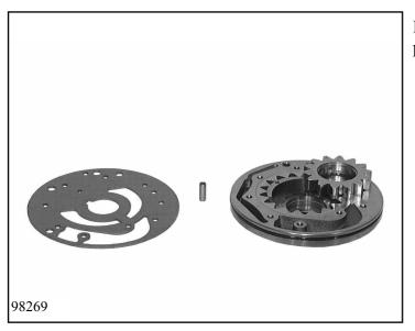
Remove the centering sleeve, intemediate plate, pump wheel and pump ring gear.
