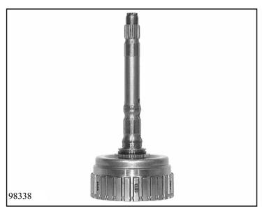
Mount 2 new rectangular-section rings 71.020 and 71.030 and new O-ring 71.150 on the input shaft.
