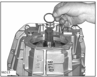
Place disc 14.050 on the parking lock wheel in the transmission housing.
