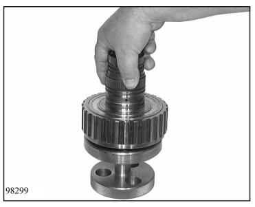
Place the complete unit on the counter support 5x46 000 577 and engage the 3 cylindrical pins of the support in the freewheel by turning.
