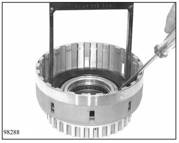
Insert cup spring 77.010/160, press down with assembly bracket 5x46 002 005 on a mandrel press and mount the split stop ring 77.010/170.
