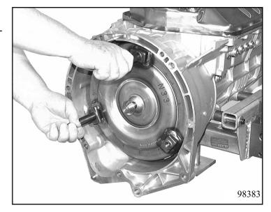
Turn the transmission by 90° and turn the converter carefully backward and forward until the pump drive journals have engaged.
