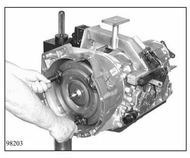
Remove the converter retaining bracket and remove the converter using two extractor handles 5x56 000 090.
