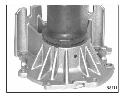
Mount the extension on holding device 5x46 002 089. Insert output flange 14.030 into the double bearing and press it in on the mandrel press using a suitable mandrel.
