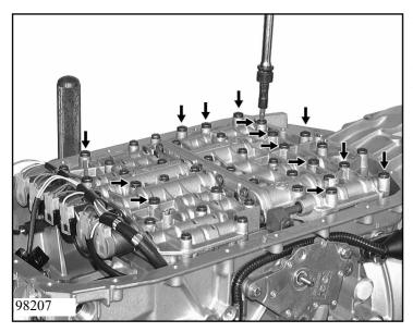
Unscrew the 14 screws with large heads as shown on the left and place the automatic control unit at an angle on the transmission housing.
