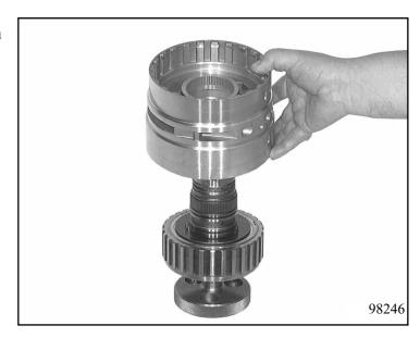
Remove snap ring, brake D. Remove the disc assembly and cup spring.
