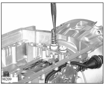
To release the sleeve of the flow control valve, press down and twist. Remove the sleeve and spring.
