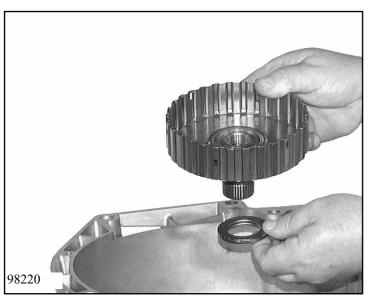
Remove the angle washer, needle cage and thrust washer.
