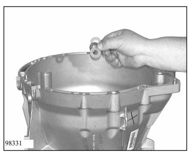
Insert thrust washer 32.200/110, axial needle cage 32.200/120 and thrust washer 32.200/130 over the journal of the intermediate shaft.
