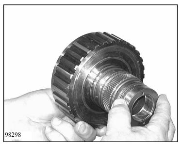
Hold the freewheel 73.100/120 firmly and press the carrier (internal sprag race) 73.100/110 into it, turning the carrier clockwise as you do so.
