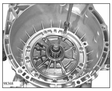
Fasten the oil supply with 9 screws 10.440 and new Usit-rings. Turn the transmission so that the oil pan is at the top.
