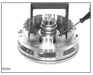
Push the cup spring down with assembly bracket 5X46 000 576. Then remove the split stop ring and the cup spring.
