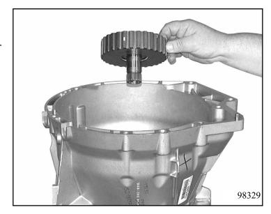
Slide angle washer 32.160/110, axial needle cage 32.160/120 and thrust washer 32.160/130 over the end of the intermediate shaft 32.180 and insert the intermediate shaft.
