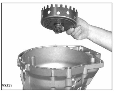
Insert sun wheel with cup 32.090 into the planet carrier.
