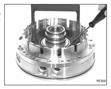
Insert complete disc assembly of brake C.
