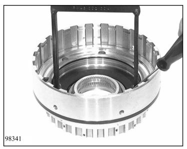
Press cup spring down with assembly device 5x46 002 004 and secure with split fixing washer 70.010/170.
