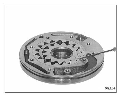
Insert centering sleeve 10.010/120 into pump casing and position intermediate plate 10.040.
