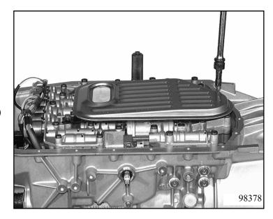
Insert 8 magnets 03.010/120 into recesses in the oil pan 03.010 - all around the oil filter intake opening.
