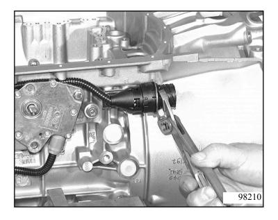
Unscrew and remove the wiring harness retaining bracket. Remove 2 retaining clips.
