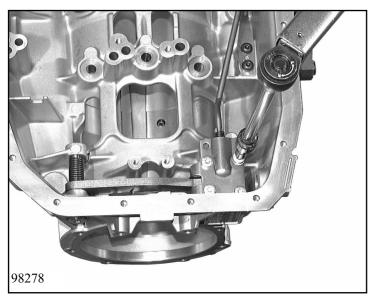
Press down the pawl and fasten guide plate 01.060 with 4 machine screws 01.080.
