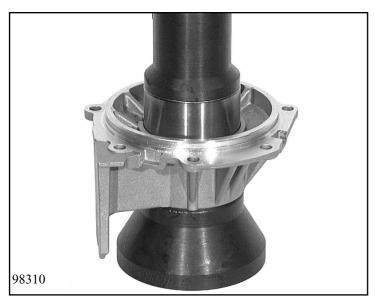
Place extension 14.010/110 on the supporting surface of the press-in device 5x46 000 760.
