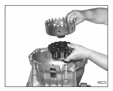
Remove the shaft with the ring gear, thrust washer, needle cage, angle washer and cup.
