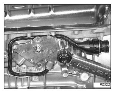
Screw 2 handles 5x56 000 090 into the converter and carefully insert the converter 22.020.
