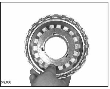
Insert cup spring 73.010/150 and fixing washer 73.090 into cylinder DG.
