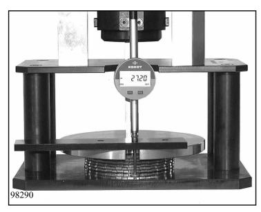
Determine thickness  $\mathbf{M}_{\mathbf{F}}$  of the brake F disc pack according to
