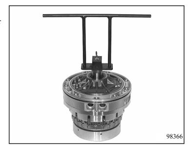
Now insert the complete unit in the transmission housing, turning it as you do so, until lined discs of clutch A and E are completely inserted, and press into end position with firm pressure on the device. At the same time, centre the oil supply over the transmission with centering pin 5x46 002 007 in such a way that the bore of the oil-supply flow control valve is in alignment with the hole in the transmission housing.
