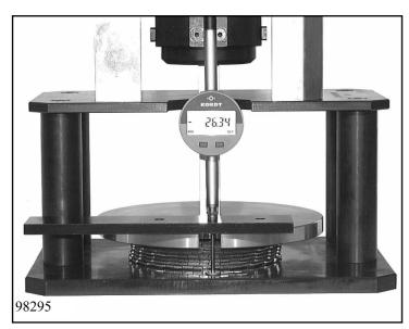
Determine thickness  $\mathbf{M}_{\mathbf{D}}$  of the brake D disc pack according to
