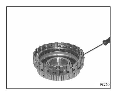
Push the cup spring down with assembly bracket 5x46 002 005 and remove the split stop ring.
