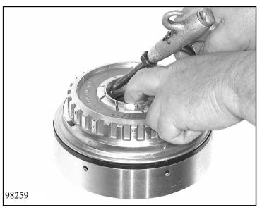
Cover 2 holes with your fingers and force the piston out with compressed air through the 3rd hole.
