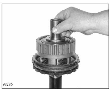
Place thrust washer 42.120/110, axial needle roller bearing 42.120/120 and angle washer 42.120/130 on planet carrier and mount the complete ring gear unit.
