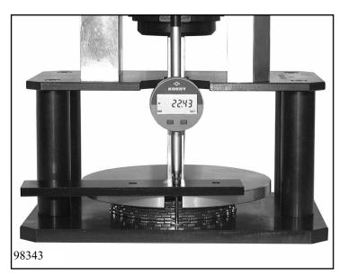
Determine thickness  $\mathbf{M}_{\mathbf{A}}$  of the clutch A disc pack according to
