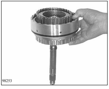
Push clutch E out of clutch A by slight pressure on the input shaft. Remove the 2 rectangular-section rings and 1 O-ring from the input shaft.
