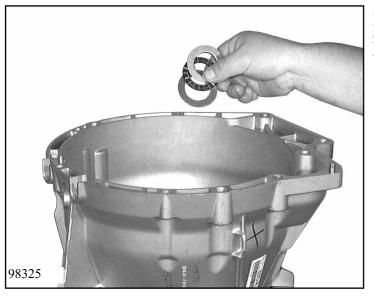
Insert thrust washer 32.060/110, axial needle roller cage 32.060/120 and angle washer 32.060/130.
