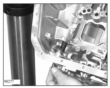
Insert pawl 01.030 and leg spring 01.040 into the transmission housing and fix them by pressing in pin 01.020. Then close the hole with screw plug 01.090.
