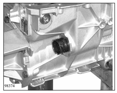
Pull 2 new O-rings 27.340/116 onto wiring harness plug 27.340. Insert plug in hole, engage guide pin in slot and fix with tab washer 27.390.
