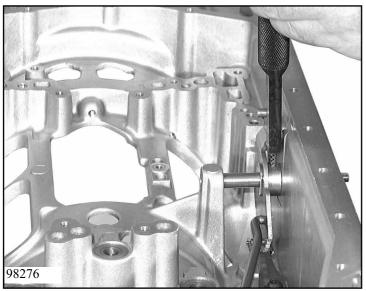
Drive new slotted pin 01.010/180 into the detent disc with driving pin 5x46 000 685.
