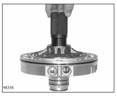
Pull new O-ring 10.360 onto oil supply and 3 new rectangular-section rings 10.370, 10.380 onto the hub of the stator shaft.
