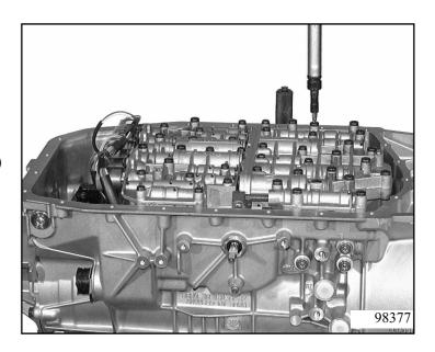
Place oil filter 27.420 on control unit with new sealing ring 27.420/020 and fasten with 2 screws 27.440.
