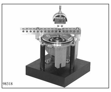
Determine dimension A between the machined surface of the extension and the hub of the output flange.
