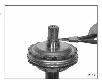
Remove the parking lock wheel. Remove the thrust washer, needle cage and angle washer from the sun wheel.
