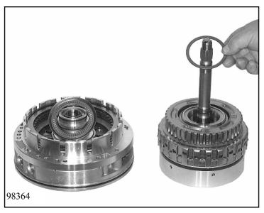
Place shim 10.400 on cylinder B. Stick angle washer/axial needle cage on stator shaft hub with a little white petroleum jelly.
