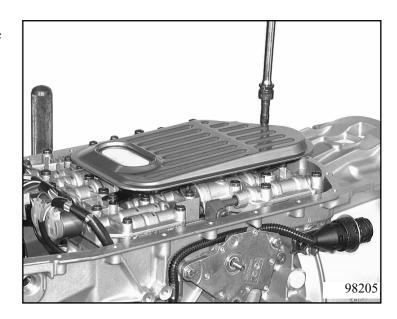
Remove retaining plate from the wiring harness plug and insert the plug into the transmission.
