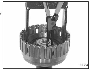
Insert complete disc assembly of clutch E, starting with spring disc 71.094. Then mount alternately steel discs 71.100 and lined discs 71.110. Mount final disc 71.120 and secure with snap ring 71.130.
