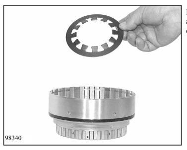
Push piston A into cylinder A 70.010/110 and insert cup spring 70.010/140 with the convex side upward.
