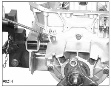
Unscrew the guide pin screw plug. Remove the guide pin and take out the pawl together with the torsion spring.
