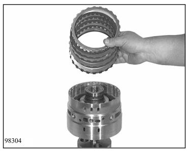
Mount 2 rectangular-section rings 73.140 on the carrier.
