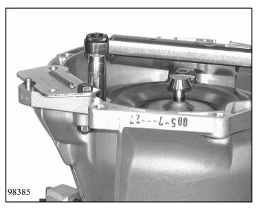
Screw the converter retaining bracket 5T95 000 099 to the converter and the transmission housing with 2 screws.
