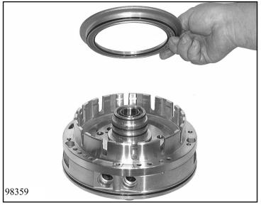
Place cylinder C 10.180 on oil supply and align.
