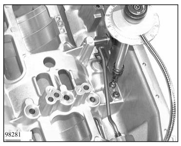
Align the roller of the detent spring at right angles to the detent disc and screw the spring tight in this position using auxiliary tool 5w04 000 583.
