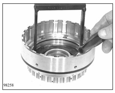
Push down the cup spring with assembly device 5x46 002 004 under a mandrel press, remove the split stop ring and cup spring.
