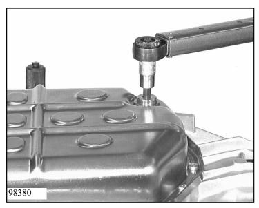
Screw new oil drain plug 03.010/130 into the oil pan.
