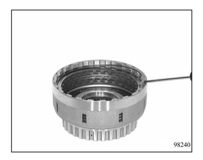
Press the cup spring down with assembly bracket 5x46 002 005 under a mandrel press and remove the split stop ring. Remove the cup spring and the pressure plate.
