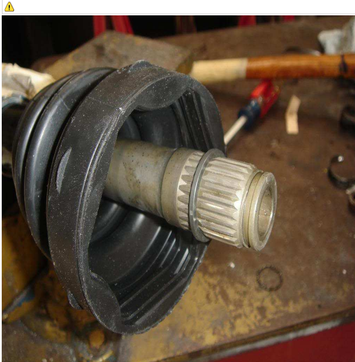
Slide the tripod and come in contact to the inner clip. Then install the outer clip
