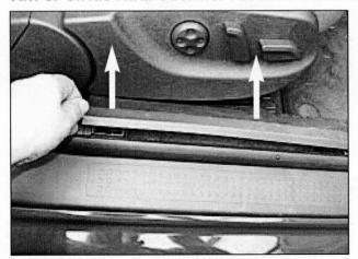
Step#15- accessing the CAN BUS connector
