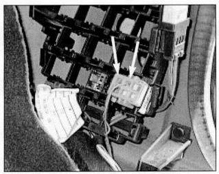
Step#17A The stock position for the Satellite radio CAN BUS connector is on the bottom right.
