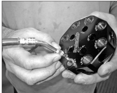
Male & female threads can be checked using the BrakeQuip Thread Gauge #BQ2100
