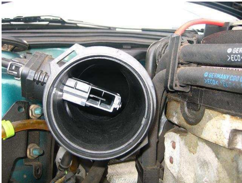
Remove this duct from the front of the airbox. This piece is pointless now that the airbox is opened up and there is no velocity sucking air from it anymore. Now, it just blocks air from the front of the airbox. I removed it completely.
