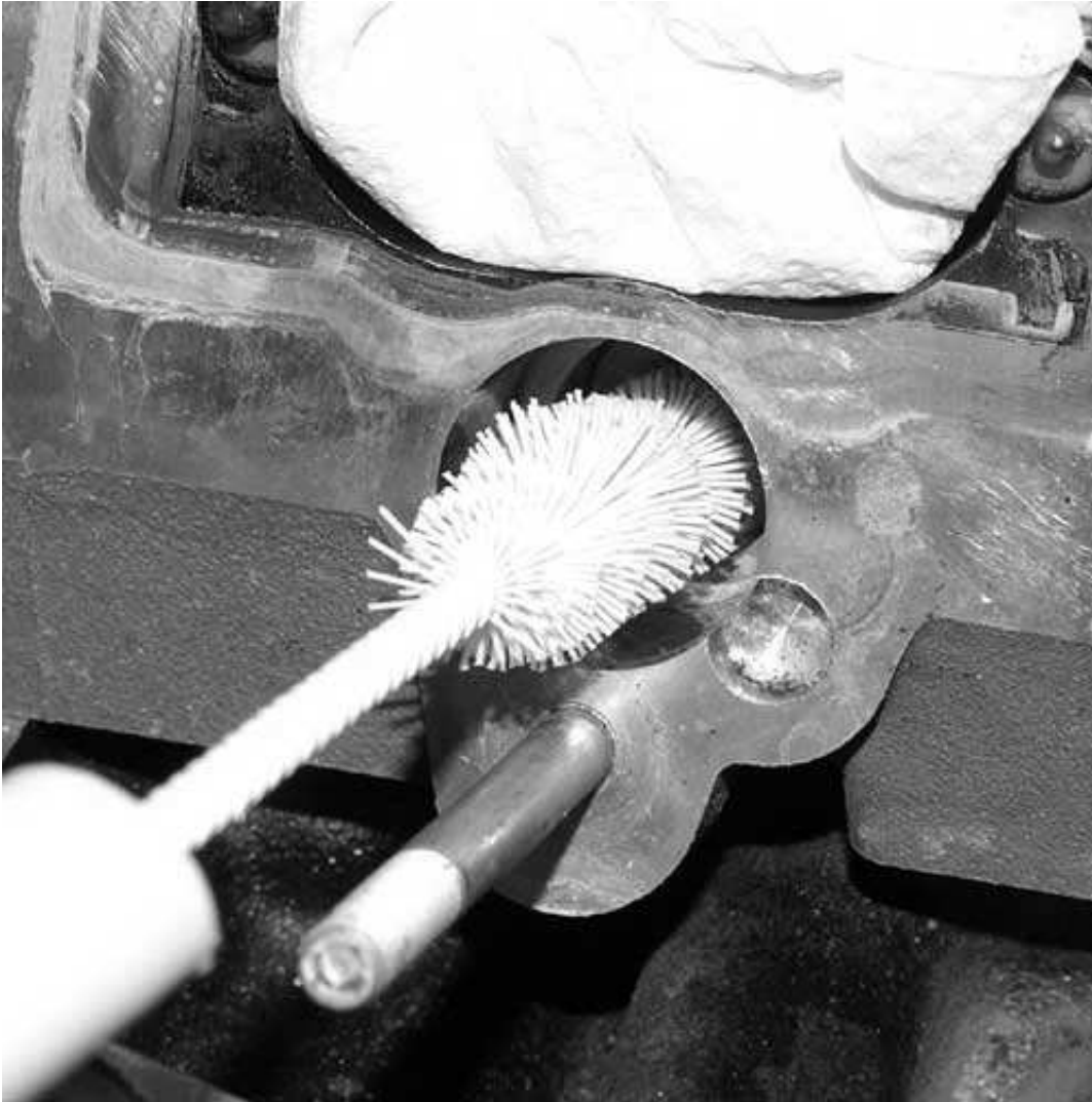
The modded bottle brush in action. Cleaning the injector ports.
