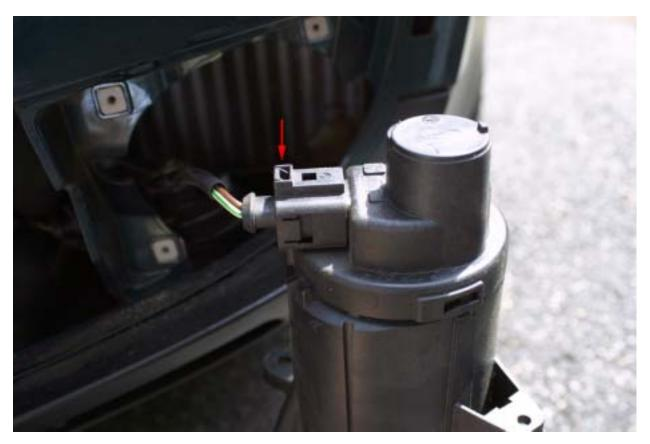
You can continue without disconnecting the wiring, or you can disconnect it by pressing down at the point shown by the arrow and pulling out the connector. Open the housing by twisting the top portion counter-clockwise.
