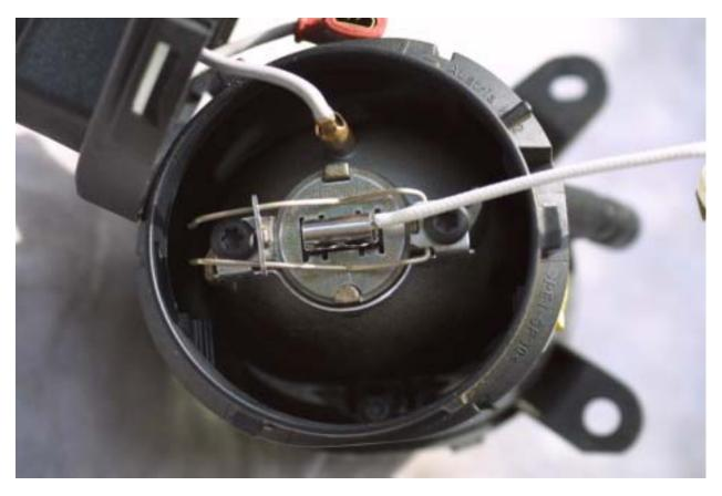
Remove the old bulb and secure the new one.
