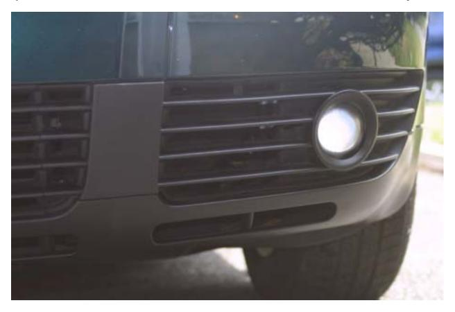
Driver's side. The foglight bulb's size is H3 at 55W. Take note that the passenger's side is the exact mirror image of the driver's side. Simply follow the same procedures for the driver's side.
