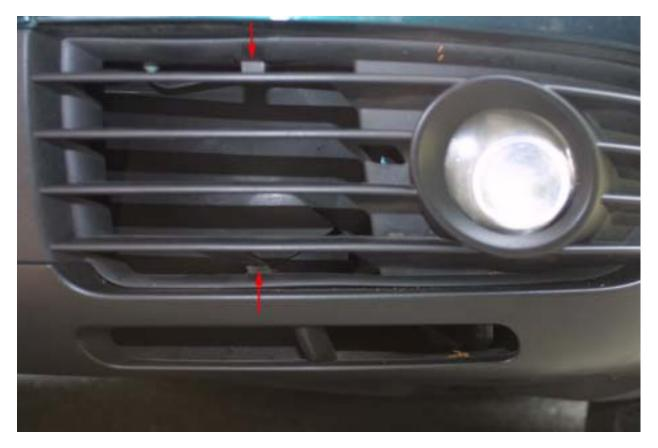
First step is to take the grill out. With your thumb and index finger on each clip, squeeze in to release and pull out.
