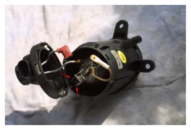
Release the clips that hold the bulb in place. Push down then out on each.
